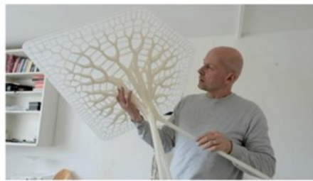
Fig. 7: Michael Pawlyn - Side table produced in PLA by 3D printing, 2014 Source: Lindsay, 2020
