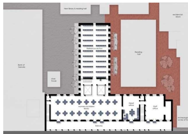
Fig. 7: First Floor Plan showing the spatial organization of spaces. Source: Drawn by the Author, 2023.
