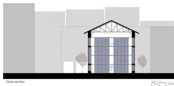
Fig. 8.1: Section of the Reference Section showing the 4-tier stacking system. Source: Drawn by the Author, 2024.
